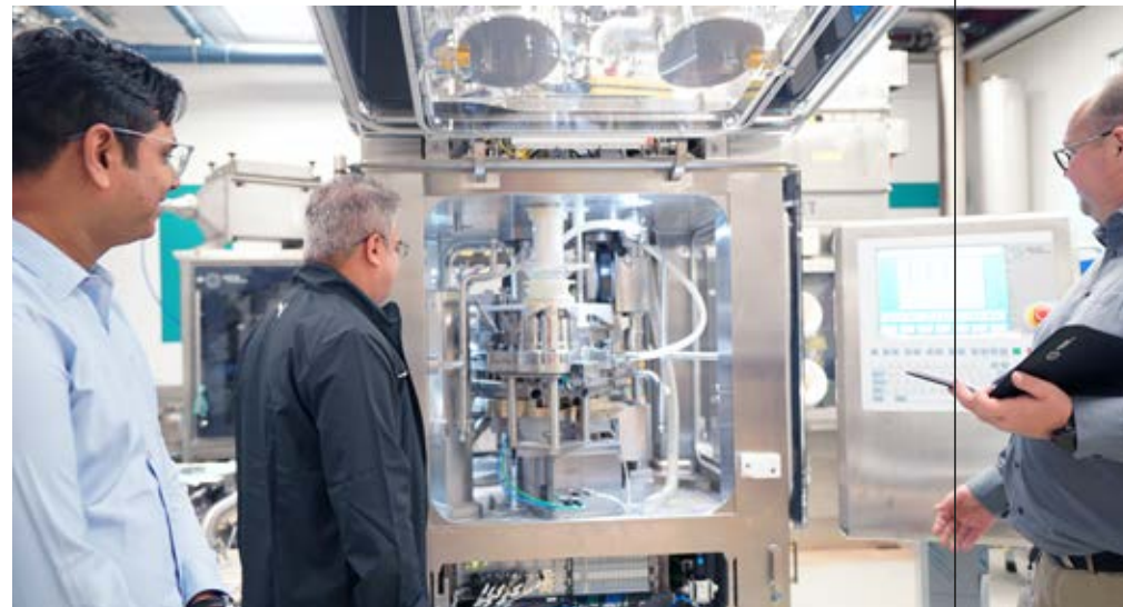
The FAT in Schwarzenbek thoroughly tested the performance of the 2090i WiP.
